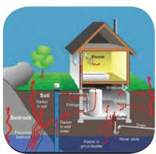
Radon gas is invisible, odourless and tasteless and enters your home through any opening where the house contacts the soil.
