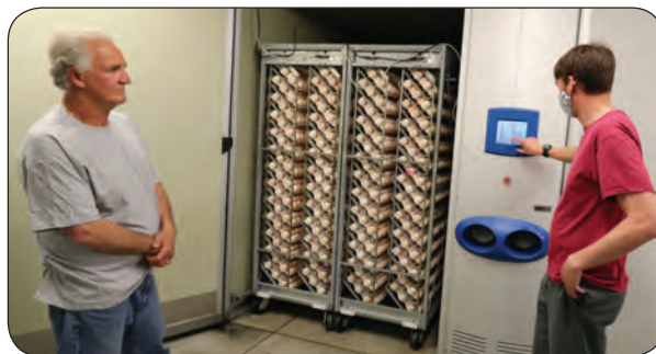
The incubators are all controlled electronically to control temperature, humidity, ventilation and egg turning cycle.
